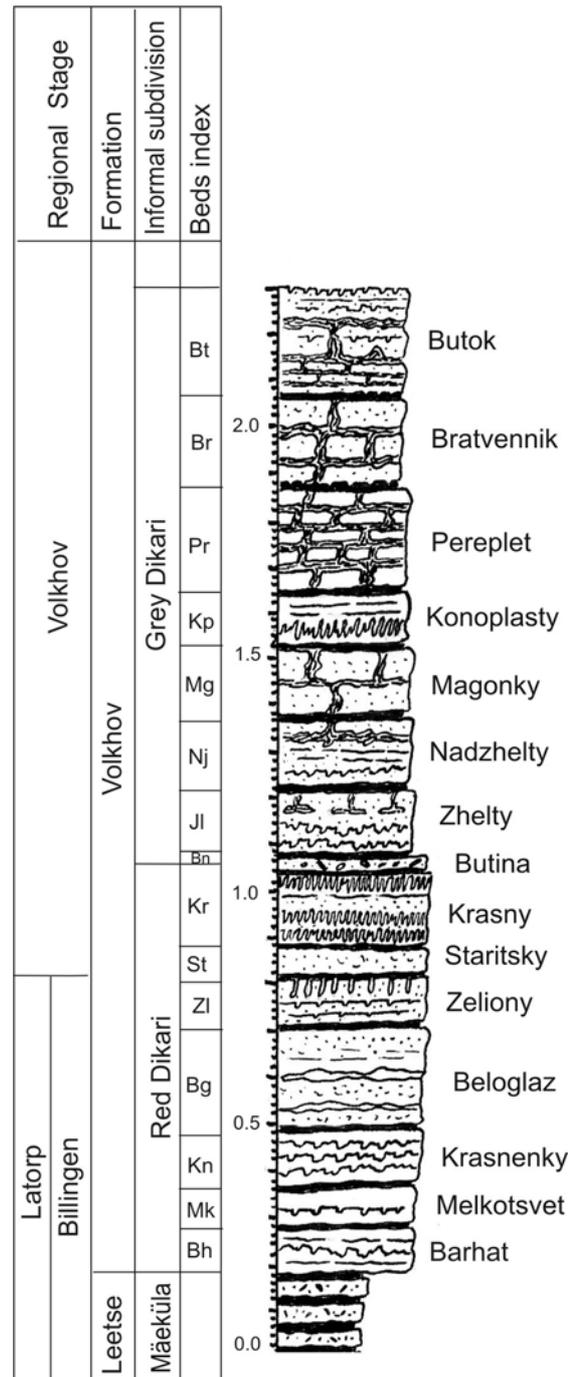
Fig. 13. The section of "Dikari Limestone" in the Putilovo Quarry.
